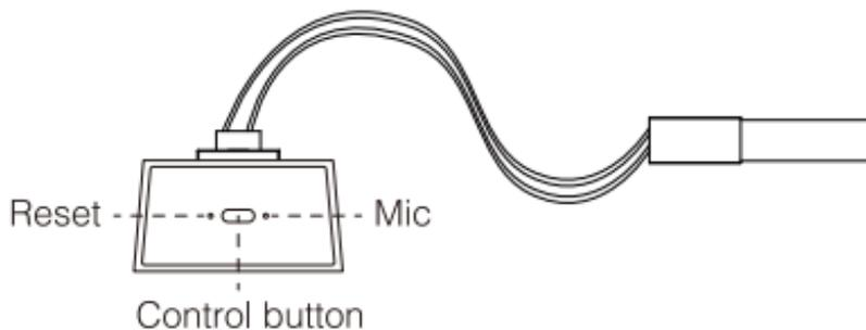
Reset method: Press and hold the reset hole until the green indicator light on the controller flashes. Release the button and the device will reboot. Wait about 10 seconds for the device to reboot successfully and complete the reset.
